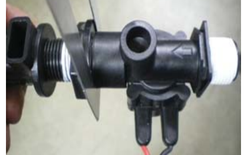
2. Unscrew float assembly at top of elbow.
